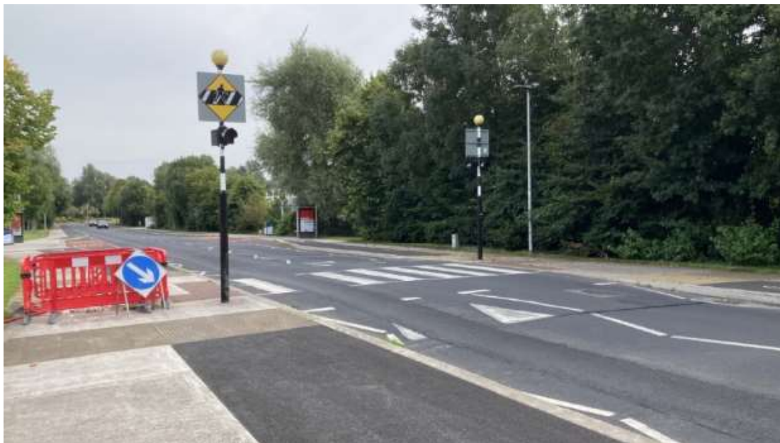
Figure 3-120: The existing Zebra crossing on Plassey Park Road proposed to be converted to a Toucan crossing
